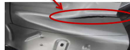
Effects of improper refining of steel
